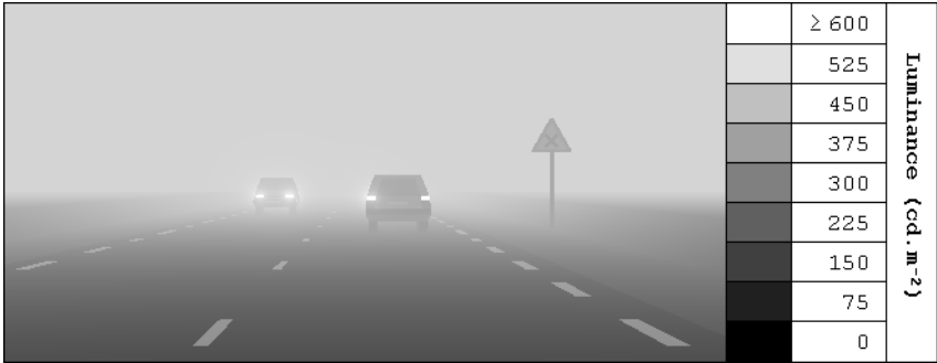
FIGURE 3. Example of iso-luminance map computed with the presented model for daytime fog: V_m = 100 m, L_r = 500 cd.m -2 (the horizontal field of view is 20°).
